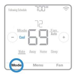
**System Mode:** The system mode is selected by tapping the bottom-left corner of the screen. Keep the system mode set to either "Heat" or "Cool." Do not select "EM Heat," this will prevent the heat pump from operating, causing the system to instead rely on costly auxiliary heating elements. Do not select "Auto," as this may cause your system to change unnecessarily between heating and cooling, increasing your heating and cooling energy use.
