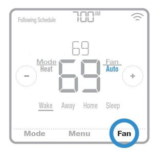
**Fan Mode:** The fan mode is selected by tapping the bottom-right corner of the screen. To view the current mode, look to the right of the temperature display, under "Fan." Keep the fan mode set to "Auto." Leaving the fan mode set to "On" will cause the fan to run continuously, wasting energy.
